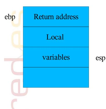
Inside a function ebs is used to keep track of the current stack value.
